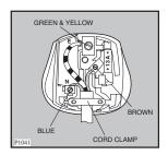
The wire coloured green and yellow must be connected to the terminal marked with the letter «E» or by the earth symbol  $\stackrel{L}{=}$  or coloured green and yellow.
